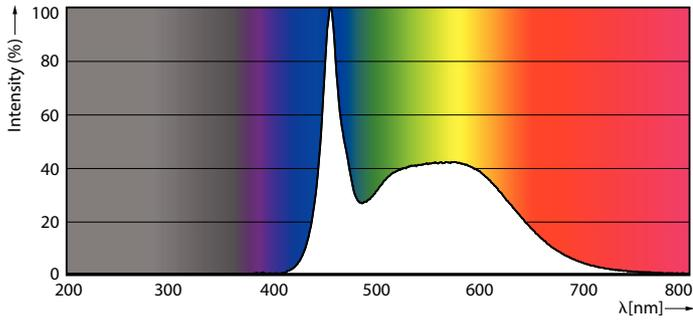
Spectral Power Distribution Colour - LEDBulb 18W E27 6500K W A23 1PF/6 MX
